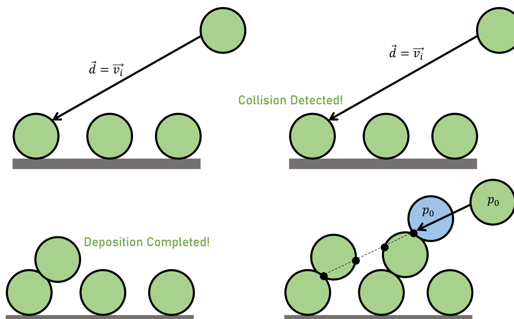
The smallest value for  $t$  is used since it allows for shadows to form between particle islands. It also causes extinction of columns in this shadowed region.
