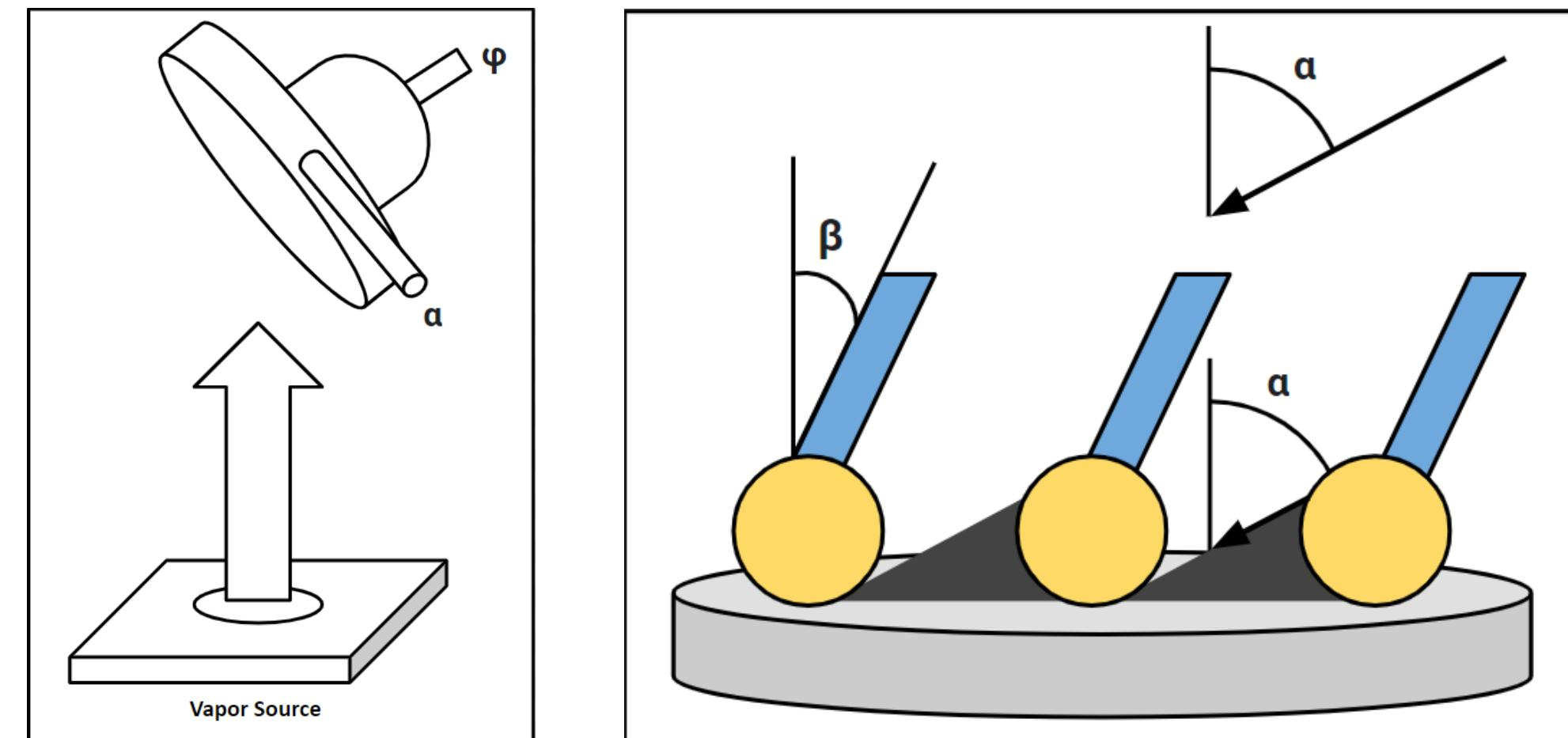
This study puts forth a way to simulate the GLAD process in a 3D environment. By applying different inputs such as incidence angle, rotation rate, deposition rate, the outcome of the simulation can be manipulated.
